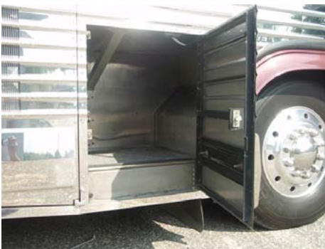
Storage compartment for hoses, spare fluids, parts
