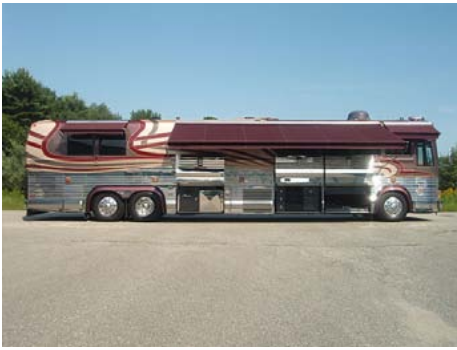
From the left, the fresh water bay, the entertainment bay and the storage bay
