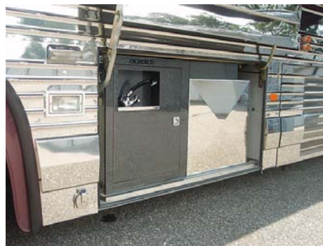
Hot and cold water faucet, fresh water tank
