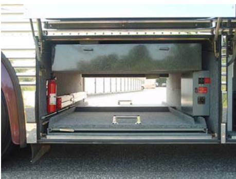
Pass through storage bay with slide-out trays, concealed drawer cabinet
