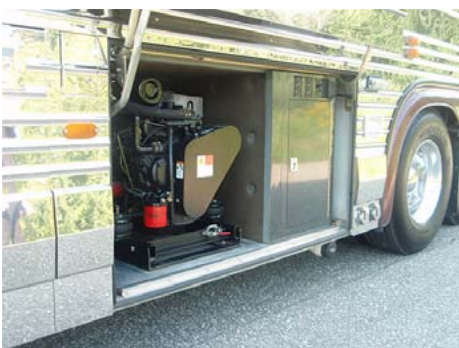
Generator bay, water bay
